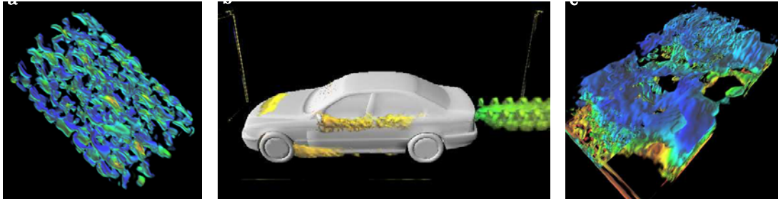
Fig. 3. Vortices extracted on the GPU. From left to right: a) DNS dataset of a flow through a cylinder filled with spheres ( 201 \times 152 \times 152 grid); b) flow around car body (RANS simulation, 301 \times 131 \times 100 grid); c) experimental data of laminar water channel ( 200 \times 40 \times 110 grid, split view for two filter kernels). Datasets courtesy LSTM, University of Erlangen, BMW AG, and IAG, University of Stuttgart.
